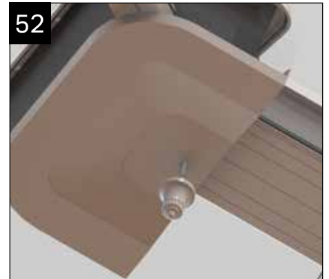
52 Offer up the internal radius end cap, use the threaded bar and the retaining boss to secure the internal cap in position. The threaded bar may require cutting to suit.
