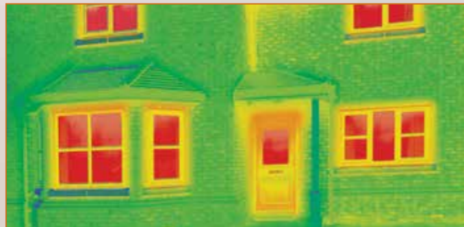
Before: Red indicates substantial heat loss through old windows.
